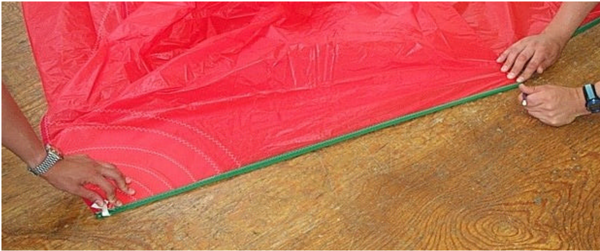
Figure 9. Finding a Spinnaker Three-quarter Leech Point
