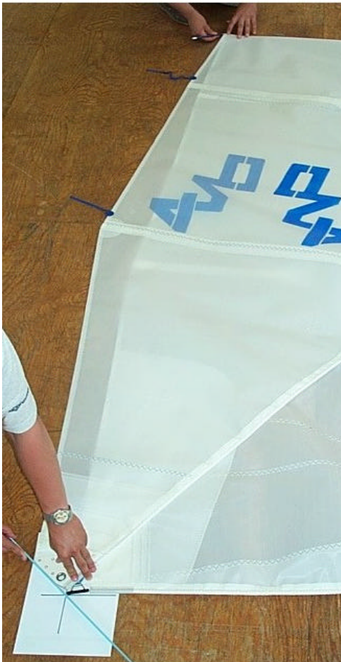
Figure 4. Finding a Mainsail Half Leech Point
