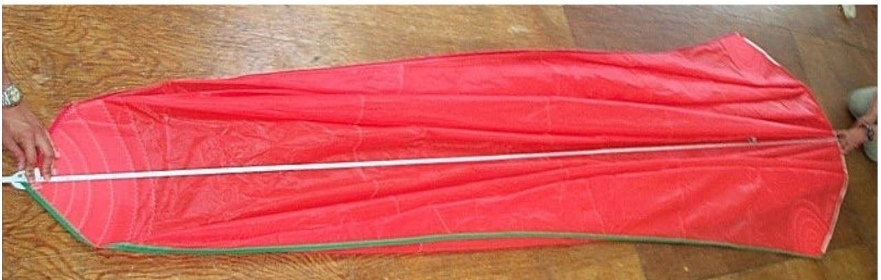
Figure 12a. Measurement of spinnaker Foot Median
