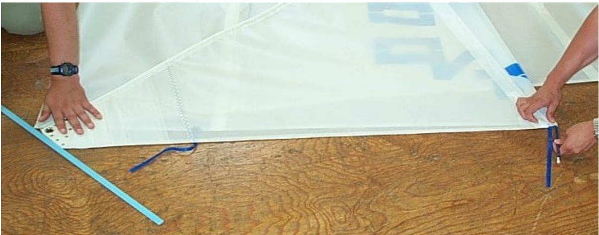
Figure 8. Finding a Mainsail Three-quarter Leech Point
