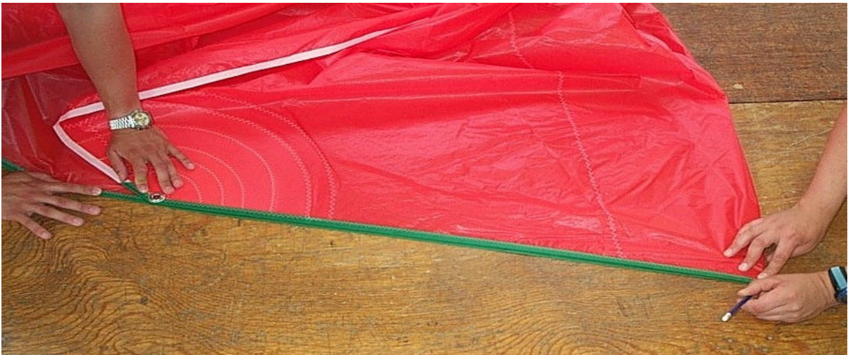
Figure 7. Finding a Spinnaker Quarter Leech Point
