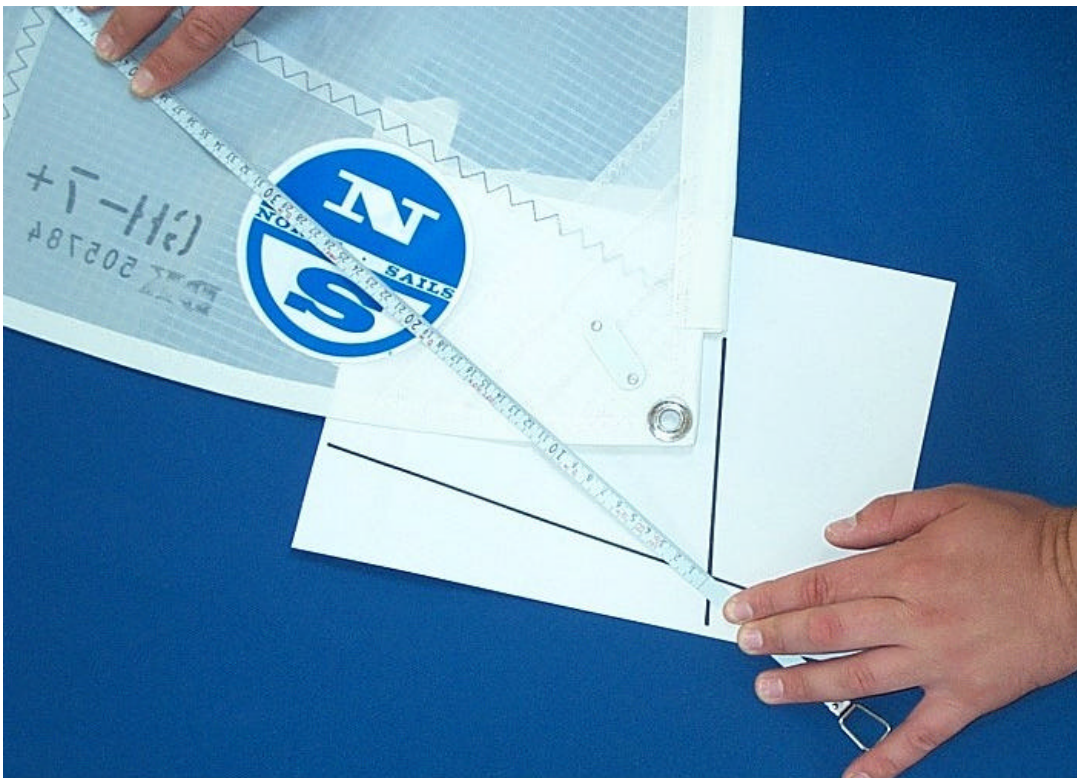
Figure 19. Measuring limit of sailmakers mark
