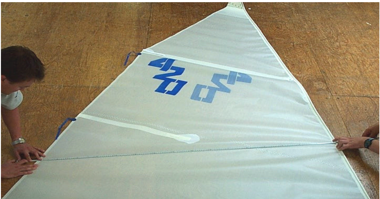
Figure 15. Mainsail Half Width
