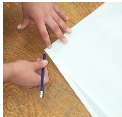
Figure 4b. Marking the edge of the sail in the fold at the leech point .
