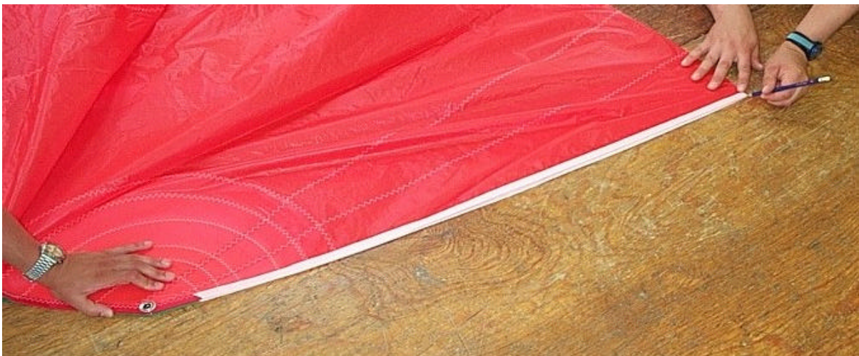
Figure 9a. Finding a Spinnaker Mid Foot Point
